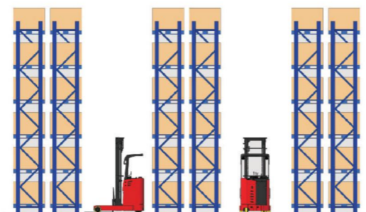
7.5 meters rack height
